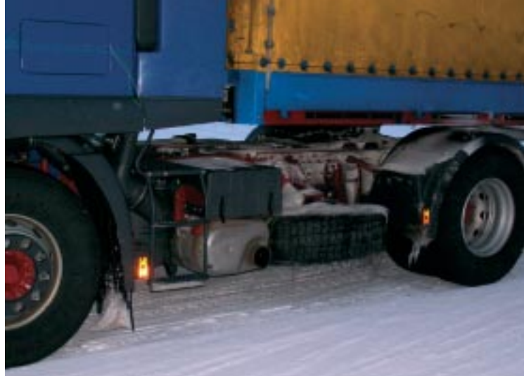
Fig.5: "WINTERTEST" of a catalyst for automotive application; the catalyst is part of the silencer system, together with a urea tank and an injection control system. By courtesy of M. Signer, IVECO Switzerland.
